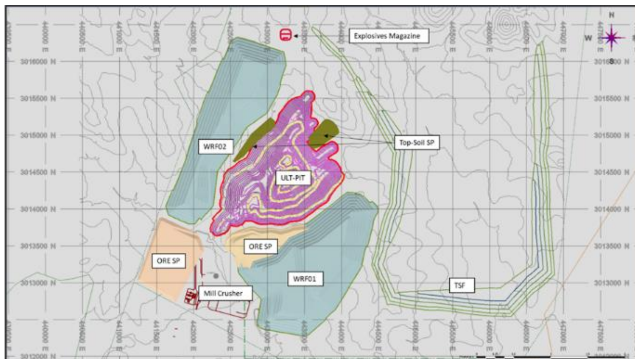
Figure 16-1: Mining Limits and General Facilities
